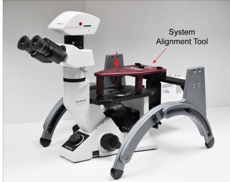
7. Looking down onto the System Alignment Tool, visually align the center opening on the Tool to the microscope objective lens (**red arrow**).
