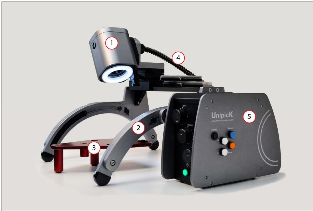
**Figure 1:** Major components of **UnipickK™**: (1) **UnipickK™** Sampler Head; (2) Universal Microscope Straddle; (3) System Alignment Tool; (4) Vacuum Line and Electrical Cables; (5) **UnipickK™** Control Box with light intensity dial (top), vacuum strength dial (middle), vacuum impulse duration dial (bottom) and DCU controls.
