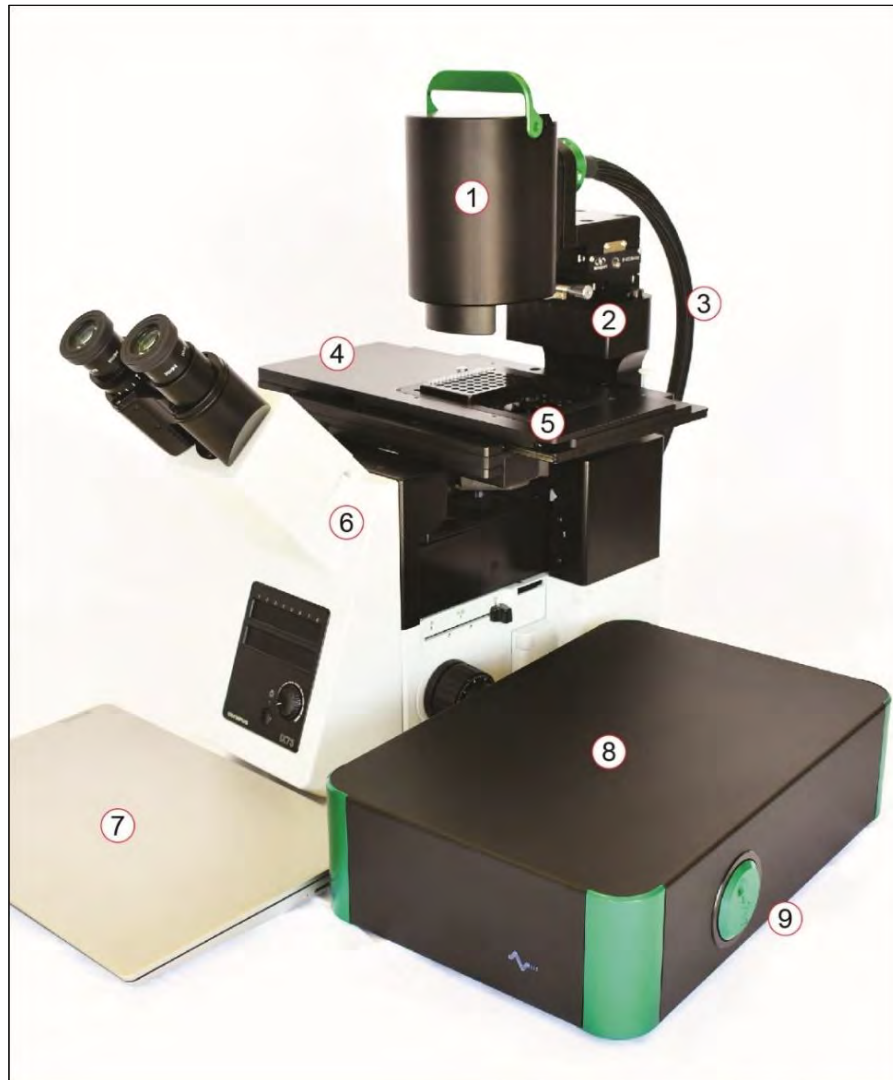
Figure 1: Major components of A-picK™ : (1) A-picK™ Sample Collection Assembly (Head); (2) Micromanipulators; (3) Vacuum and Pressure Line and Electrical Cables; (4) Motorized stage; (5) Universal Sample Holder; (6) Olympus IX73 Inverted Microscope; (7) Personal computer with PIKCELLS™ software for process control; (8) A-picK™ Control Box; (9) Side panel of A-picK™ Control Box with the green Calibration wheel.
